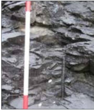
Figure 69: FID5 - Detail of drilled shot hole in quarry face.
